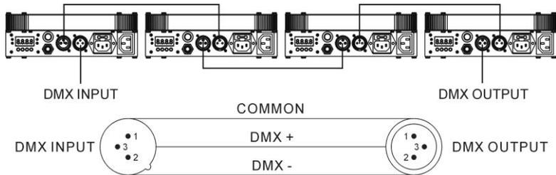
Termination reduces signal errors and to avoid signal transmission problems and interference. It is always advisable to connect a DMX terminal.
