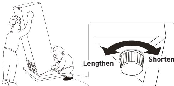
If the unit is not level, the doors and magnetic seal alignments will not be covered properly
