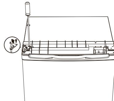
8. Put the top cover and fix it with 2 screws on the back.
