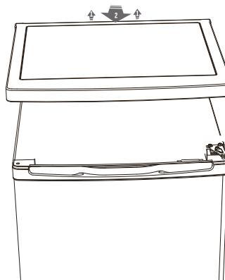
3. Unscrew top hinge and then remove door and place it on a soft pad to avoid scratch.
