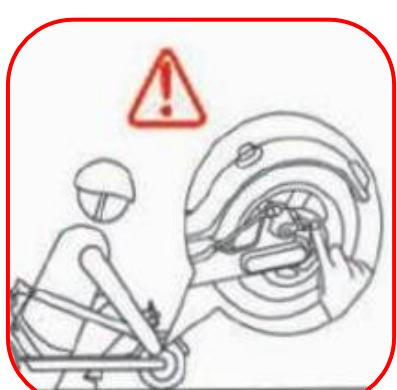
Do not touch the disc brakes after using your scooter, these parts can be hot after a long ride.
