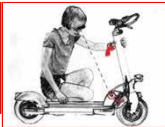
Then pull the folding handle and lower the stem towards the tray of your scooter. Once lowered to its maximum, return the safety buckle to its original position.
