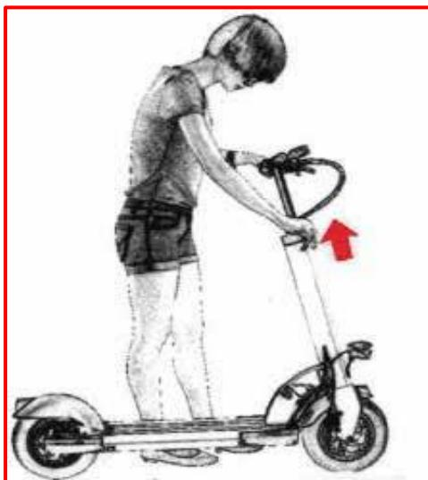
Adjust the size of your handlebars by loosening the clamp on the stem. Be careful not to exceed the height limit indicated. Check that your handlebars are stable and that the clamp is tight.
