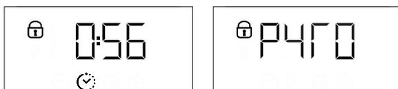
Once the cycle has been completed, the door remains locked until the temperature inside the oven has returned to a safe level. Air the room during and after running the Pyro cycle.
