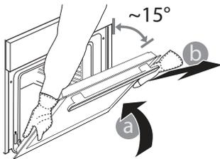
2. Close the door as much as you can. Take a firm hold of the door with both hands – do not hold it by the handle. Simply remove the door by continuing to close it while pulling it upwards at the same time until it is
