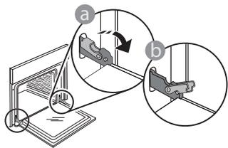
1. To remove the door, open it fully and lower the catches until they are in the unlock position.
