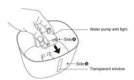
The correct installation direction of the water pump: Side @ facing Side 6
