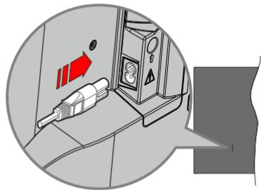
Plug one end (the two-hole plug) of the supplied detachable power cord into the power cord inlet on the rear side of the TV as shown above. Then plug the other end of the power cord into the mains socket outlet.
